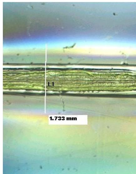
Figure 7. Polarized light microscopy photograph of Clearweld heat affect zone in polycarbonate [4].
