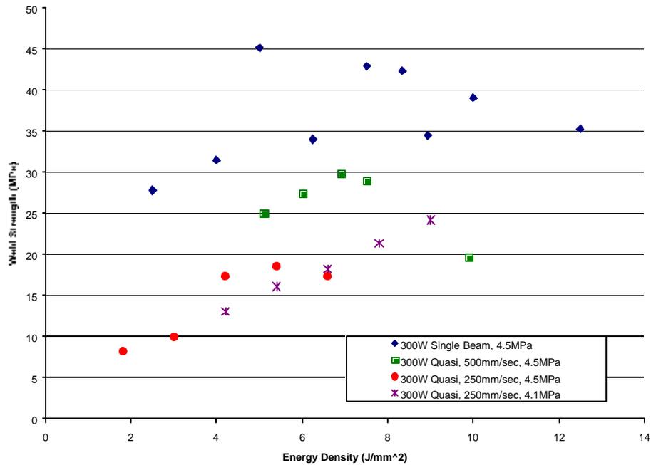
Figure 6. Quasi-simultaneous versus single beam laser welding of acrylic.
