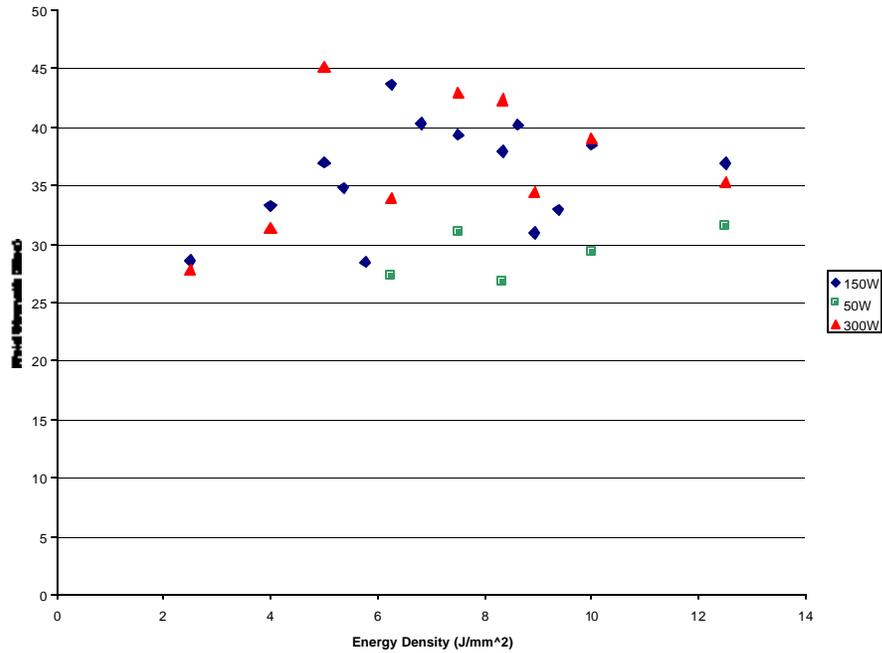
Figure 4. Effect of power on acrylic weld strengths.
