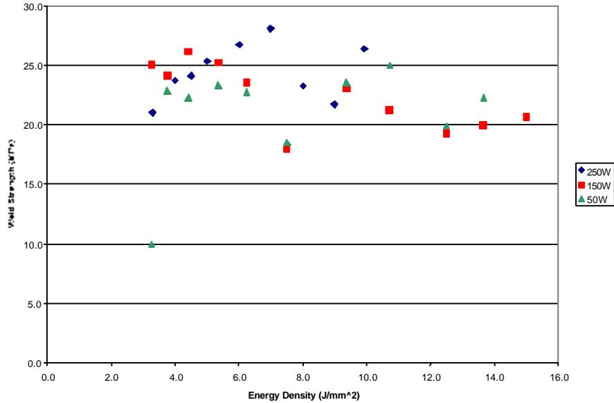
Figure 3. Effect of welding parameters on polypropylene.
