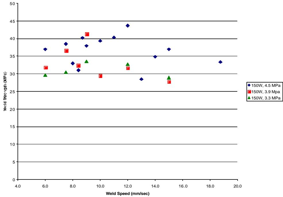
Figure 5. Effect of clamping pressure on acrylic weld strengths.
