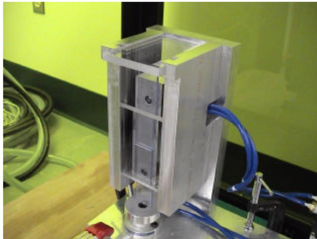
Figure 1. Clamping system for Clearwelded butt joints.
