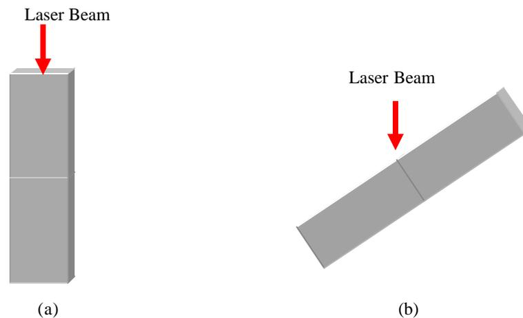
Figure 2. Orientation of Acrylic (a) and polypropylene (b) with respect to the laser beam.
